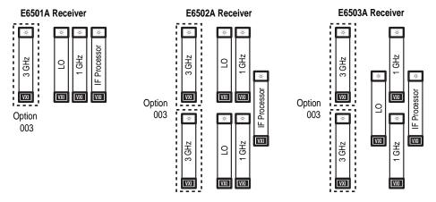
Agilent E6501A, E6502A, and E6503A VXI receivers each cover the 2 MHz to 1000 MHz frequency range. Option 003 extends the frequency range to 3000 MHz.
