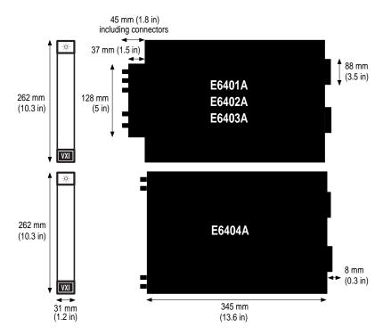
Dimensions of VXI modules included in the Agilent E65XXA receivers.
